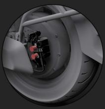
3 calipers for front, 2 calipers for rear.
